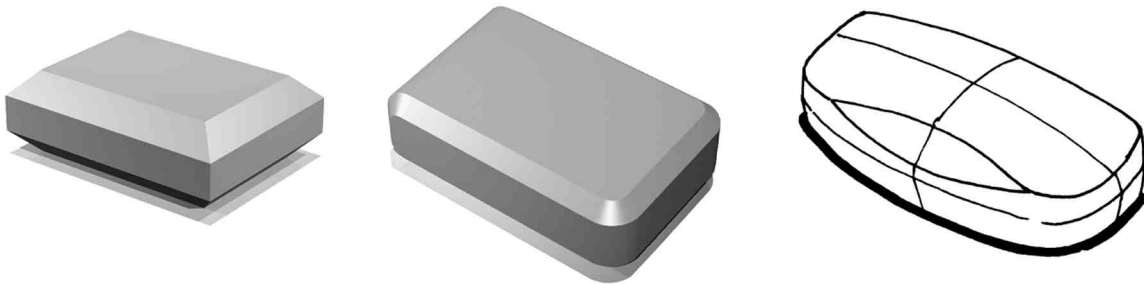
Figure 6: adding surfaces by chamfering left starting from a basic geometrical volume, in the middle starting from a first generation design, right adding a surface by making a cut.
